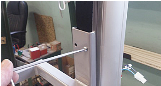
5. Assemble fork and let the screws penetrate holes of the seat belt.
