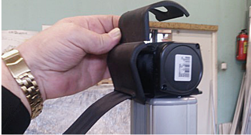
1. Open the lid of the belt. Pull out the belt from the reel until attachment holes are visible to enable inserting screws in place.
